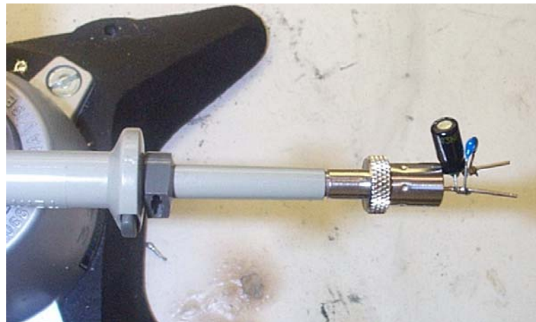
Figure 14 – Oscilloscope Probe with Probe Master 5125BA BNC Adapter. (Modified with wires for probe ground for ripple measurement, and two parallel decoupling capacitors added)
