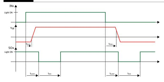
Figure 1 Driver Behavior and Status Feedback in Normal Operation
