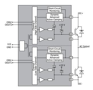
The 2SP0430V2 is a dual channel plug-and-play gate driver for PrimePACK™ 3+ power modules. The gate driver is available in different variants, which all provide reinforced isolation for all primary-side signals:
