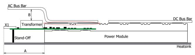
Figure 5 2SP0430V Mounted on PrimePACK<sup>TM</sup>3+ Power Module showing Relevant Distances to the Surrounding..
