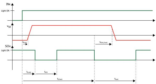
Figure 1 Driver Behavior and Status Feedback under Fault Condition
