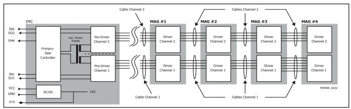
Figure 3. Functional Block Diagram of 2SILT1200T2A0C with 4 2SMLT0220D2C0C MAGs.
