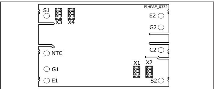
Figure 2. Pin Configuration of 2SMLT0220D2C0C.
