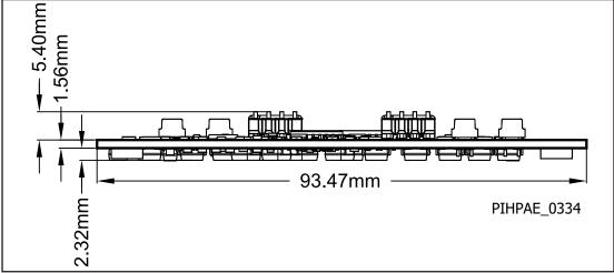
Figure 6. Side View of 2SMLT0220D2C0C.
