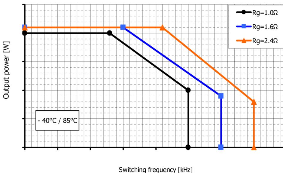
Fig. 3: Permissible output power vs. switching frequency
