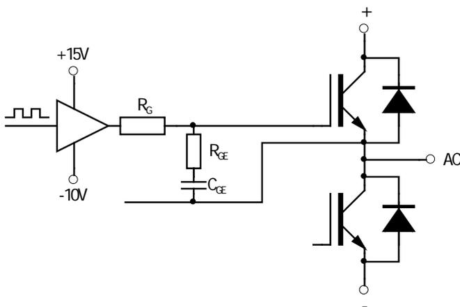
Fig. 1: Gate drive with additional RC element
