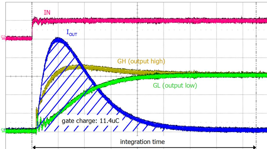
Fig. 2: Gate charge measurement by integrating the output current over time
