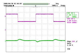
Figure 20 – Transient Response, 230 VAC, 50%-100%-50% Load Step.
