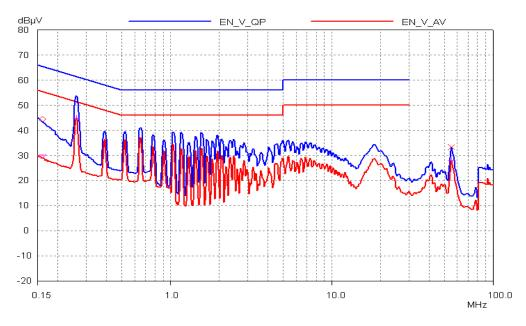
Figure 31 - Conducted EMI, Maximum Steady-state Load, 230 VAC, 60 Hz, EN55022 B Limits.
