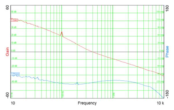
**Figure 29** – Gain-phase Plot, 230 VAC, Maximum Steady-state Load. Vertical Scale: Gain = 10 dB/div, Phase = 30 °/div. Crossover Frequency = 400 Hz, Phase Margin = 60°.
