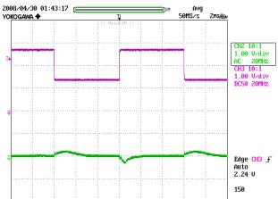
Figure 18 – Transient Response, 90 VAC, 50%-100%-50% Load Step.
