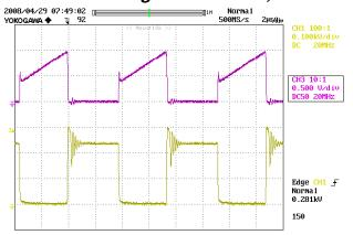
Figure 12 – 90 VAC, Full Load. Upper:  $I_{DRAIN}$ , 0.5 A/div. Lower:  $V_{DRAIN}$ , 100 V, 2  $\mu$ s/div.
