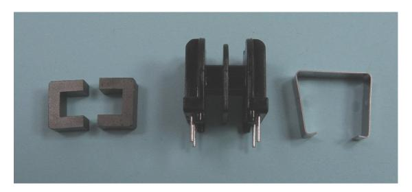
Figure Showing Core, Bobbin and Core Clip
