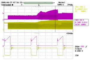
Figure 16 – 90 VAC Input and Maximum Load. Upper:  $I_{DRAIN}$ , 0.5 A/div. Lower:  $V_{DRAIN}$ , 200 V. 2 ms/div and 2  $\mu$ s /div.
