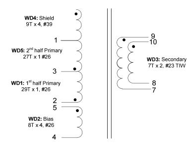
Figure 5 – Transformer Electrical Diagram.
