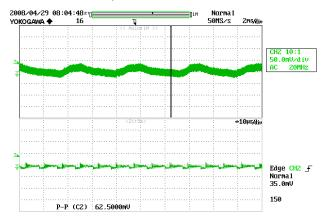
**Figure 26** – Ripple, 230 VAC, Full Load. 2 ms, 50 mV/div.
