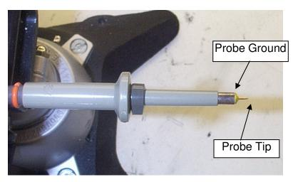
Figure 22 - Oscilloscope Probe Prepared for Ripple Measurement. (End Cap and Ground Lead Removed)
