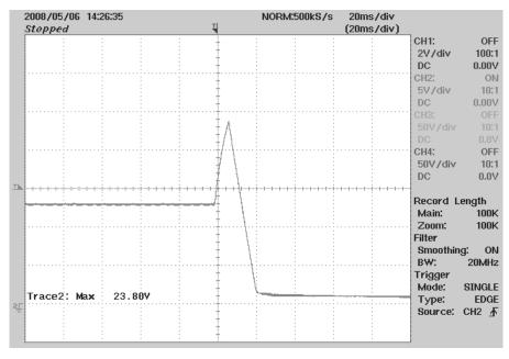
Figure 21 – Output Voltage, Open-loop Test. Vin = 264 VAC.
