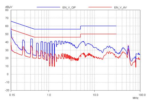
Figure 30 - Conducted EMI, Maximum Steady-state Load, 115 VAC, 60 Hz, EN55022 B Limits.
