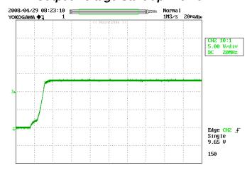
Figure 14 – Start-up Profile, 115 VAC 5 V, 20 ms/div. Resistive Load.
