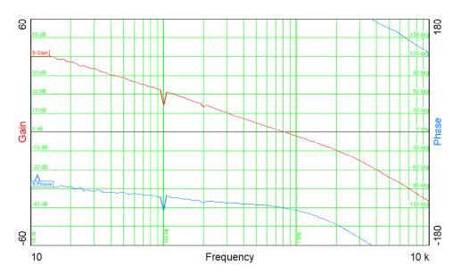
Figure 27 – Gain-phase Plot, 90 VAC, Maximum Steady-state Load. Vertical Scale: Gain = 10 dB/div, Phase = 30 °/div. Crossover Frequency = 800 Hz, Phase Margin = 60°.
