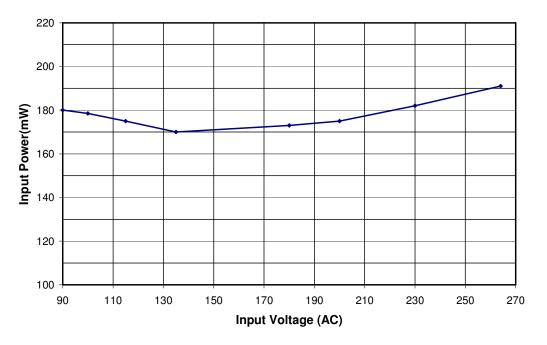
**Figure 8** – Zero Load Input Power vs. Input Line Voltage, Room Temperature.
