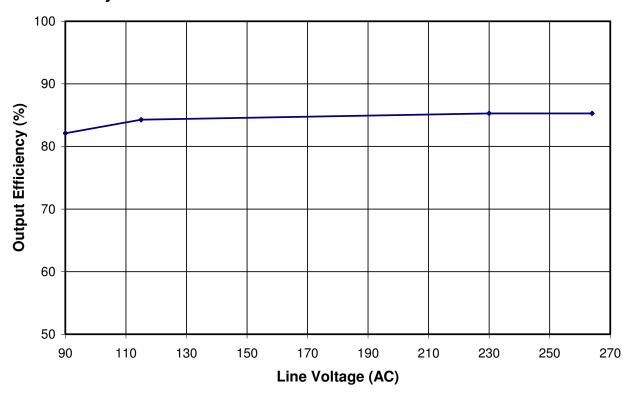
**Figure 7** – Efficiency vs. Input Voltage, Room Temperature.
