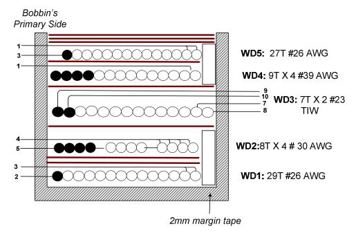
Figure 6 – Transformer Build Diagram.
