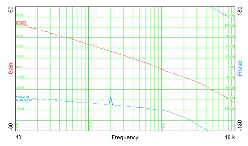
**Figure 28** – Gain-phase Plot, 115 VAC, Maximum Steady-state Load. Vertical Scale: Gain = 10 dB/div, Phase = 30 °/div. Crossover Frequency = 1.0 kHz, Phase Margin = 60°.
