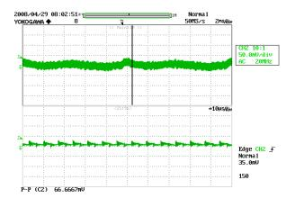
**Figure 24** – Ripple, 90 VAC, Full Load. 2 ms, 50 mV/div.
