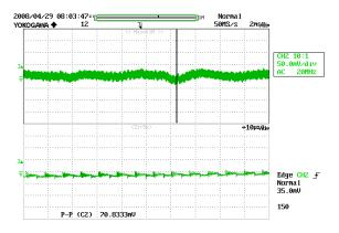
**Figure 25** – Ripple, 115 VAC, Full Load. 2 ms, 50 mV/div.
