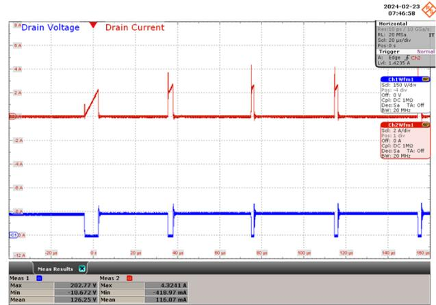
**Figure 75** – 100 VAC, 42 V LED Load.
