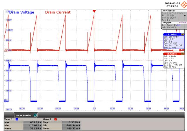
**Figure 73** – 277 VAC, 42 V LED Load.
