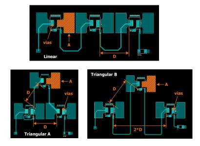
Figure 3 Linear and Triangle A / B Device Configurations (Bottom Layer)
