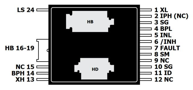
Figure 1 BridgeSwitch InSOP-24C Bottom View
