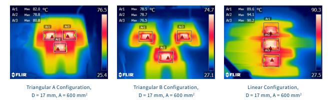
Figure 5 Thermal Device Scans of Triangular vs. Linear Configurations and a 1.5 W Package Dissipation
