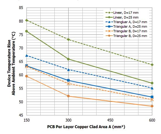
Figure 4 Average Device Temperature Rise vs. Configuration, per Layer Copper Clad Area, and Device Distance
