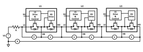
Figure 2 Test Setup Circuit Diagram
